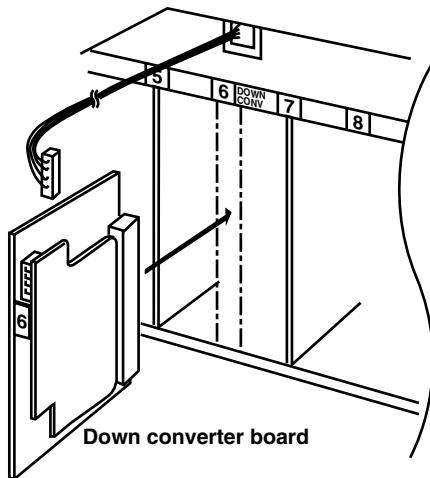
④ Insert the other end of the cable into the connector on the board itself.
